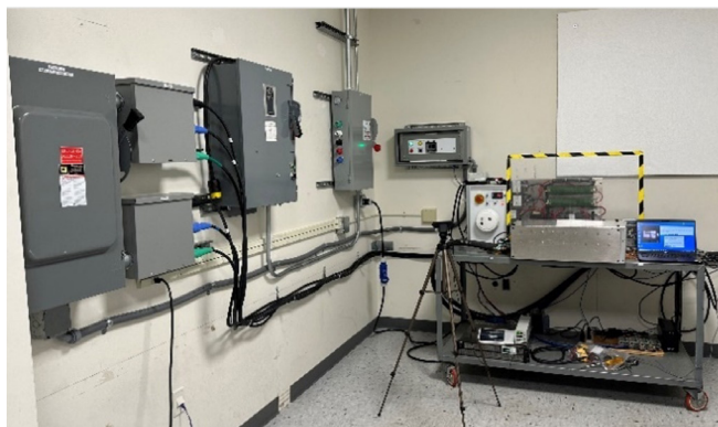
FIGURE 2. SD SSR Endurance Tester
