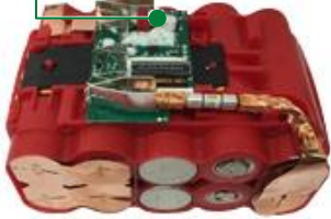
Li-ion rechargeable 20700 Cell 3.6 V / 3.15 Ah, 5S2P configuration
